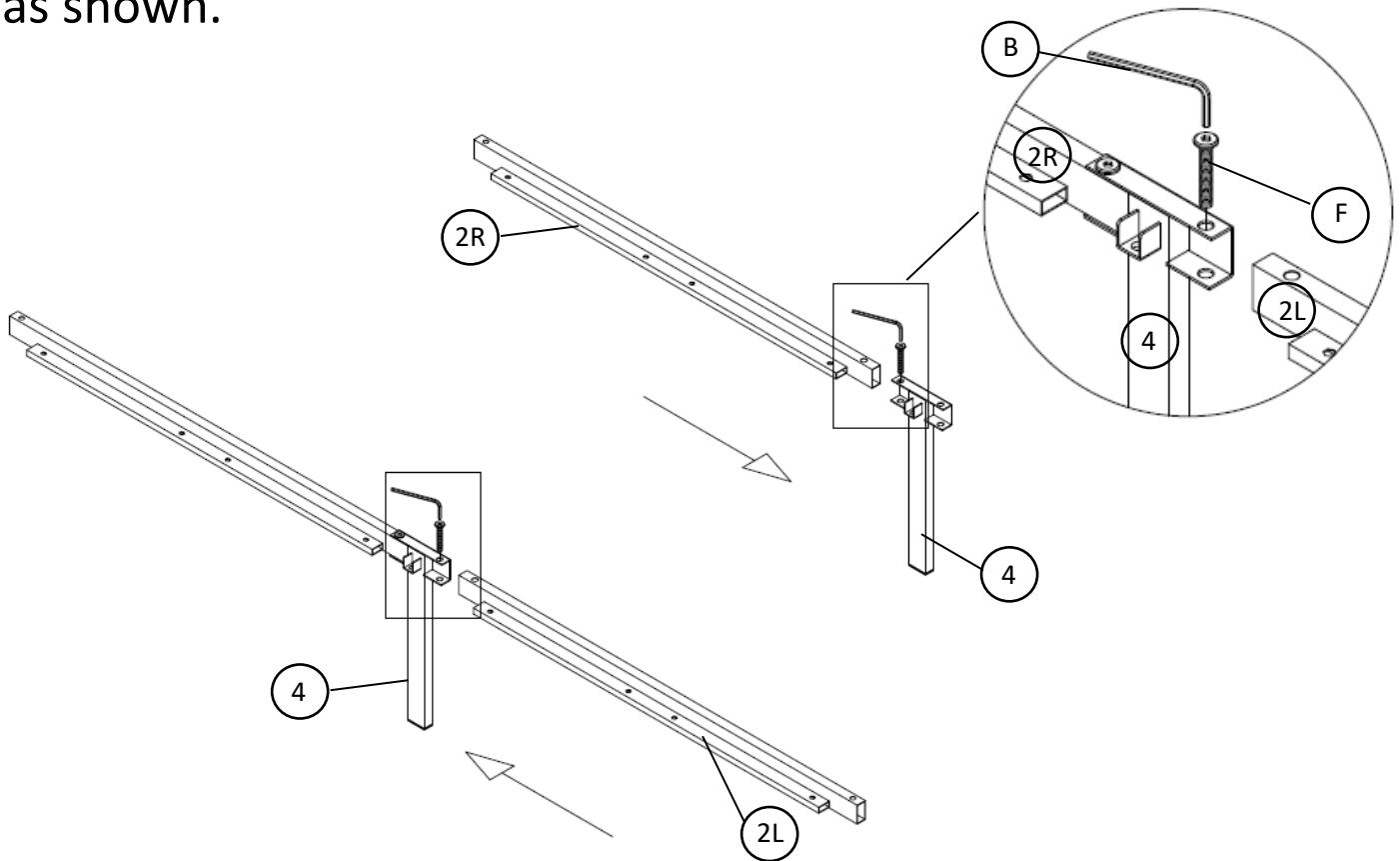
STEP 2 : Attach (1) to (2) by using (D) with Allen Key M5 (B) as shown.
